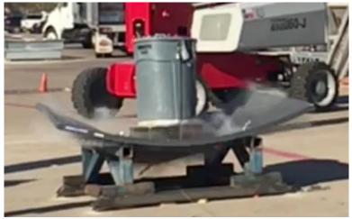
Photo No. 1 Impact and Test Stand Configuration
